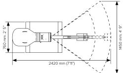
NOTE: The Digger/Grabber can be altered for swing and digging depth.
